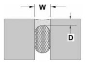
EXPANSION JOINTS - The minimum width and depth of any sealant application should be 1/4" x 1/4" (6 mm x 6 mm).
